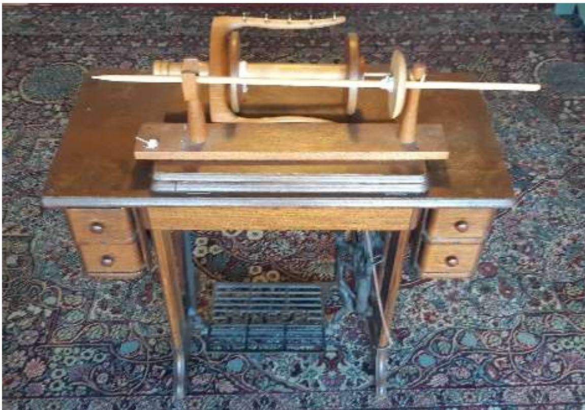
Figure 6 Singer treadle sewing machine with the sewing machine removed and the 'Salish Head' traditional spindle showing how the spindle transitioned to the Salish head. (Photo by author)
