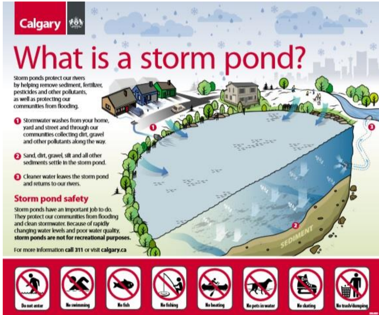
Figure 1. What is a Stormpond? Reprinted from Storm Drainage System FAQ, In www.Calgary.ca , n.d., Retrieved August 24, 2018, from http://www.calgary.ca/UEP . Copyright 2018 by The City of Calgary. Reproduced with permission.
